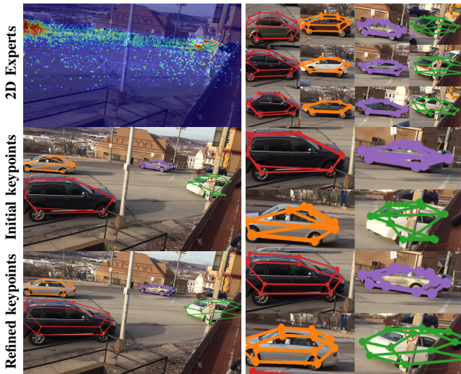
Fig. 6: Examples of keypoint refinement via 2D longitudinal self-supervision. First row: Visualization of 2D experts. The heatmaps show frequency of 2D experts being used to refine other instances. 2D experts are used mostly at image border, occluded or far away places. The vehicle patches show the top three nearest neighbors retrieved from expert pool (good keypoints predicted by initial detector), which have very similar shape and pose to the refined instance; Second row: Initial erroneous keypoints from detector; Third row: Refined keypoints after 2D longitudinal self-supervision.
