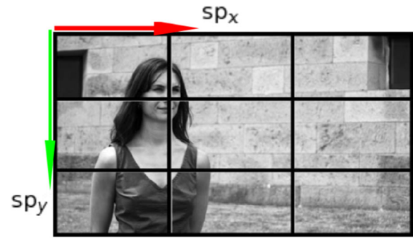
FIGURE 7 Desired screen position of the actor projection, defined by parameters: sp_x, sp_y \in [0, 1] . Typically the user uses one-third of the screen to set the actor's position or centers the actor on the frame (Bowen & Thompson, 2013) [Color figure can be viewed at wileyonlinelibrary.com ]
