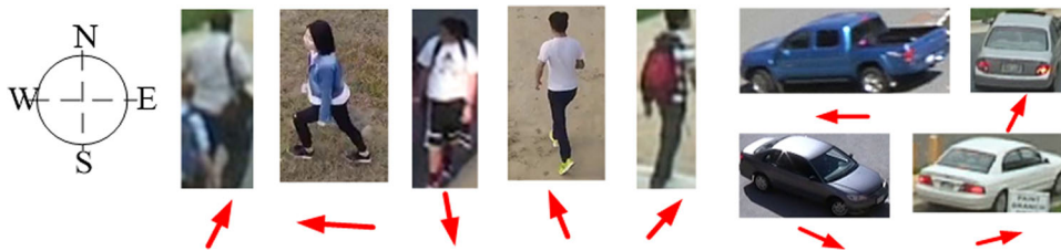
FIGURE 8 Example of actor bounding boxes and their respective heading angles \psi_a in image space. Given the images, our objective is to predict the heading direction, shown as red arrows [Color figure can be viewed at wileyonlinelibrary.com ]
