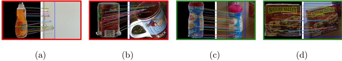
Figure 5.3: (a, b): False positives from the base detector filtered by FLOWVERIFY; (c, d): True positives from the base detector accepted by FLOWVERIFY.
