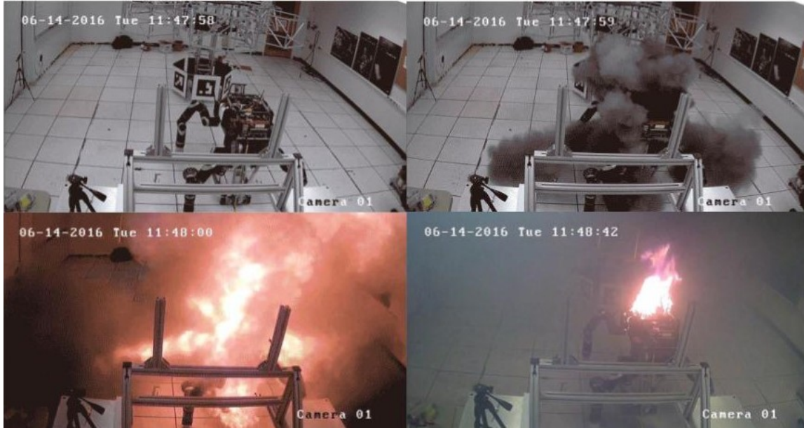
Figure 3.2: The 2016 RoboSimian battery fire caused by thermal runaway that destroyed most of the robot body during unsupervised charging, an example of storage volatility in Li-Ion batteries, adapted from [42].
