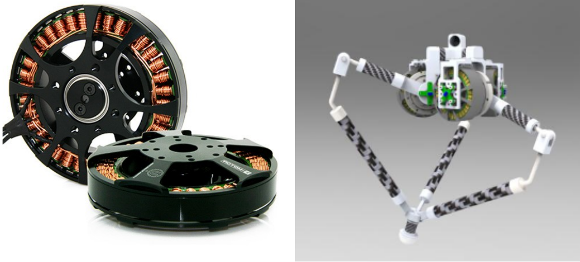
Figure 3.10: A Tiger Motor designed for direct drive applications, from [66] (left), and the GOAT leg which used three direct drive actuators to power a parallel leg mechanism for dynamic movement with proprioception, from [32] (right).
