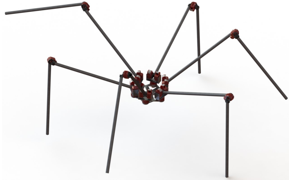
Figure 4.2: A render of the original Hebi-6 design with doubled hip modules and no onboard electronics shown.
