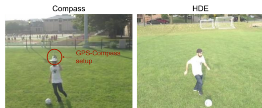
Fig. 9: Comparison of resulting drone images taken using a compass-GPS setup and visual HDE. The use of a compass and GPS module significantly decrease image aesthetics, and proves to be impractical in most real-life applications for a drone cinematographer. Meanwhile, the visual HDE requires less hardware, is simpler, and allows more complex and constraint-free actor motions.
