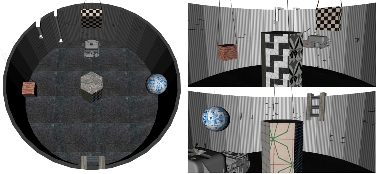
Figure 4.16: Simulation environment with HAUV model pictured. It is a metrically accurate rendering of the real-world tank environment, with targets of different geometries suspended. The central object is hexagonal piling-like structure.
