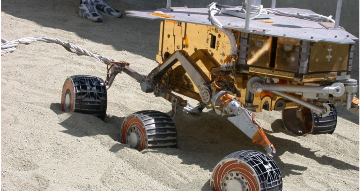
Figure 1.1: Spirit and Opportunity rover analogue being tested driving through deep soil [1]
