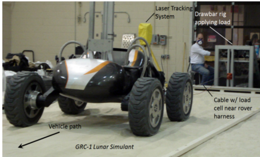
Figure 1.6: Test setup with scarab rover and cable to apply constant load [5]
