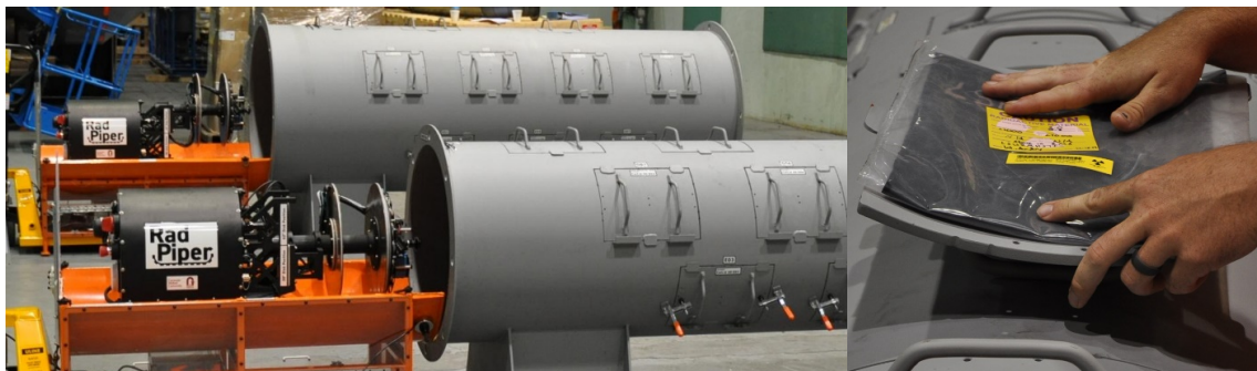
Fig. 10. (Left) RadPiper deploying into 30- and 42-inch PCAMS test pipes. (Right) Technician securing a known U-235 source in a removable test pipe panel.
