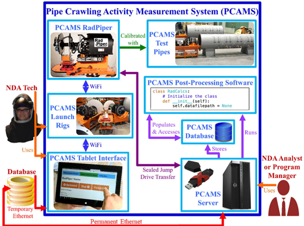
Fig. 3. PCAMS system overview. NDA technicians remotely deploy the pre-calibrated robot on its launch rig via a wireless tablet request loaded from the site database. Data collected by the robot is transferred via jump drive to the PCAMS server that databases the information, runs auto-analysis and reporting software, and allows NDA analysts and managers to edit and approve the report. Upon approval, PCAMS NDA results are directly exported to the site database.
