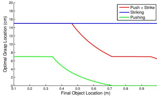
Figure 6. The plot shows how the optimal grasp of the hammer varies on the following actions. As the final object location increases, the object had to be pushed further from its initial 0.1m position. The length of the handle limits the grasp location to 15cm.
