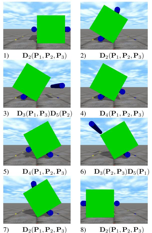
Figure 3. The images show the system in different stages of the two-handed tumbling procedure. The two blue cylinders are the hands  $P_1$  and  $P_2$ . The green object is the box  $P_3$ . Under each image is the step number, and the allocation of tokens to the continuous systems.
