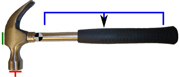
Figure 5. The hammer  $P_9$  used in the experiment. The blue marking defines the part of the handle that affords grasping. The red marking defines the impact point used for striking objects. The green marking is the region of the hammer's head used for pushing objects. The black and gray circle indicates the center of mass.
