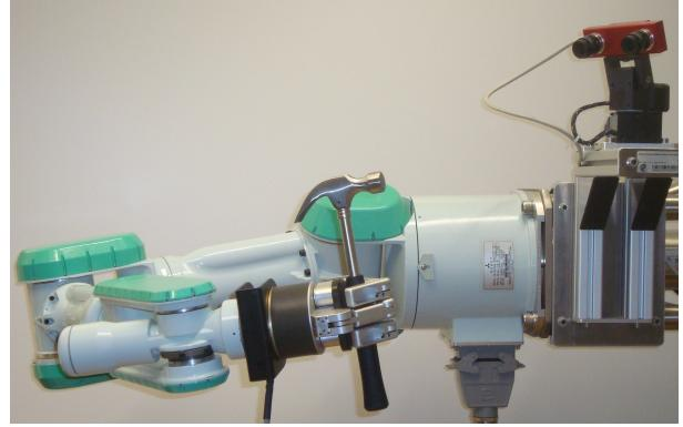
Figure 1. Robot with an optimal grasp of hammer for subsequent pushing and striking actions.
