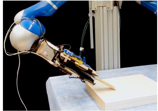
Fig. 6. Scraping task on an elevated surface after five policy updates. The robot controls the height such that the spatula gently touches the surface.
