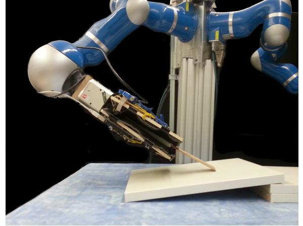
Fig. 1. Robot performing a gentle scraping task using tactile feedback.
