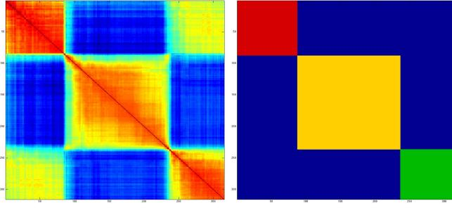
Fig. 3. Similarity matrix heat-map (left) and spectral clustering (right) of tactile images of the scraping task. *Clusters:* red (top left) - moving towards the table, yellow (center) - scraping along the table surface, green (bottom right) - moving back to the initial position
