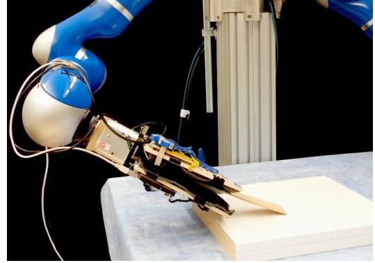
Fig. 5. Scraping task on an elevated surface before any policy updates. The robot goes too far down, resulting in a larger force and a smaller angle to the surface.
