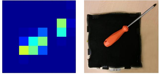
Fig. 2. Tactile image of a screwdriver handle (left) acquired from a tactile matrix array (right).
