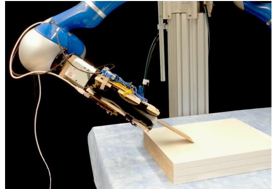
Fig. 7. Scraping task on a surface elevated to 7.5 cm and using a policy learned on a 5cm elevation. The robot still controls its height correctly.
