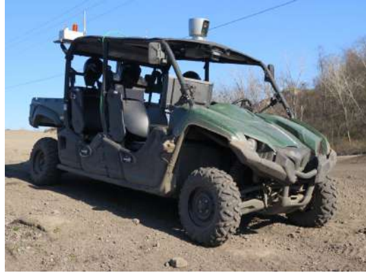
Fig. 1 Our Autonomous All-Terrain Vehicle (ATV). The two main sensors, a spinning 3D LiDAR and a stereo camera, can be seen on the vehicle roof.
