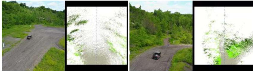
Fig. 11 Aerial action shots of autonomous off-road driving in our testing site. The left-hand side shows the vehicle, and the right-hand side shows the semantic map as seen by the vehicle. Video will be made available on the project page.
