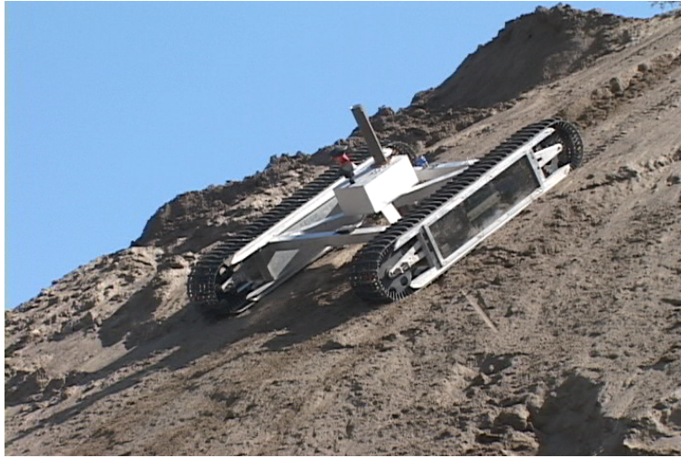
Figure 13: Icebreaker rover with actuated plow engaged.
