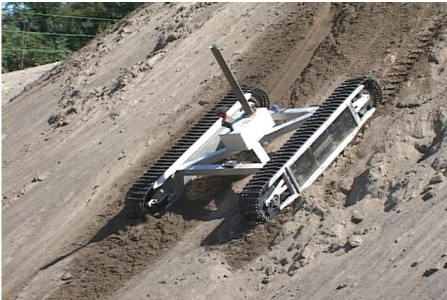
Figure 15: Example of fluid-like flows of the soil surface layer forming during a turn execution. Flows are seen as darker soil underneath the tracks of the rover prototype.
