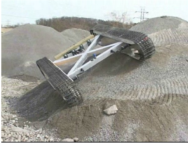
Figure 9: The prototype rover is traversing mounds of loose slag material, showing significant sideslip.
