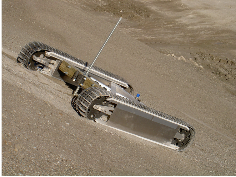
Figure 12: Initial plow experiment dragging a threaded rod to set various depths of penetration.
