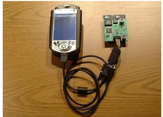
Figure 1: Each participant in the CTF game is equipped with the hardware shown above. Left: the iPAQ H3650 handheld and BackPAQ interface sleeve. The BackPAQ provides several I/O options including an accelerometer, camera and 802.11 wireless communication. Right: the Cricket listener (indoor location sensor) provides an estimate of the user's global position.
