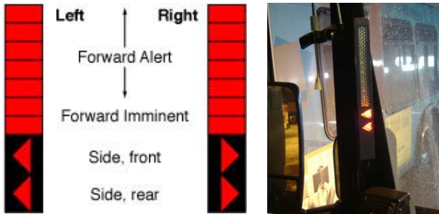
Fig. 3. Integrated DVI. The forward LEDs grow downwards with threat level and “aim” at threat. The triangles point towards the relevant mirrors. Bars are mounted on the pillars of the driver’s forward window.
