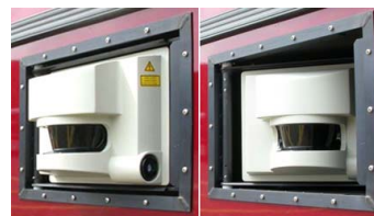
Fig. 6. Side laser extended (operation) and retracted (flinch, fail, or off).
