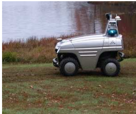
Fig. 1. Grizzly is a navigation test-bed built upon a commercially available All Terrain Vehicle (ATV). It uses two laser scanners to perceive the shape of the world. The vehicle is equipped with differential GPS and a six-axis inertial measurement unit that provides accurate attitude.
