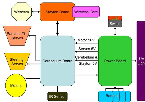
Fig. 4. PER electronics schematic.
