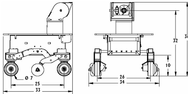
Fig. 3. PER dimensions in centimeters.
