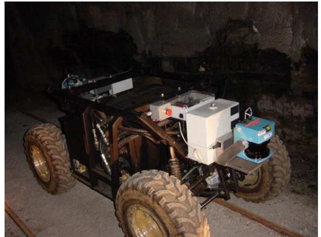
Fig. 1. Groundhog, our current robotic mine mapping platform
