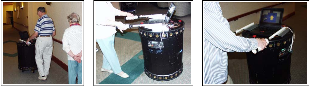
Figure 4: (a) The robotic walker, as it escorts an elderly person. (b) The haptic interface for controlling the walker. (c) The walker’s display provides simple directions (in form of an arrow) as to where to move for the present target location.
