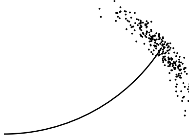
Figure 3.5: Samples drawn from the probabilistic motion model.
