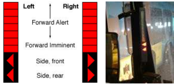
Figure 11: The DVI. On the left is a schematic of the arrangement of the LEDs. On the right is an image of one of the LED bars with only the side warning triangles lit.
