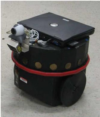
Fig. 1. Hardware environment in use for the 2004 edition of *Mobile Robot Programming Laboratory*: Nomad Scout with Dell laptop equipped with a PCMCIA wireless card and a Logitech USB webcam. The camera is fixed on the magnet support and facing forward. The circles on the side of the robot are its sonars.
