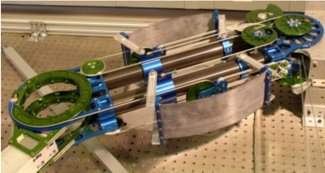
Figure 1: An Actuator with Mechanically Adjustable Series Compliance (AMASC)
