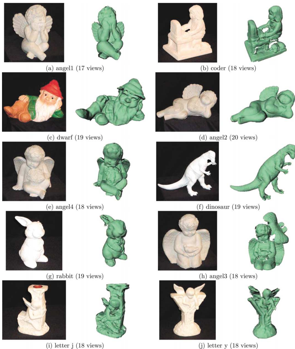
Fig. 11. Photographs of the 10 test objects (first and third columns) and the resulting 3D models (second and fourth columns). All of the objects were correctly reconstructed except angel3, which contains one error.
