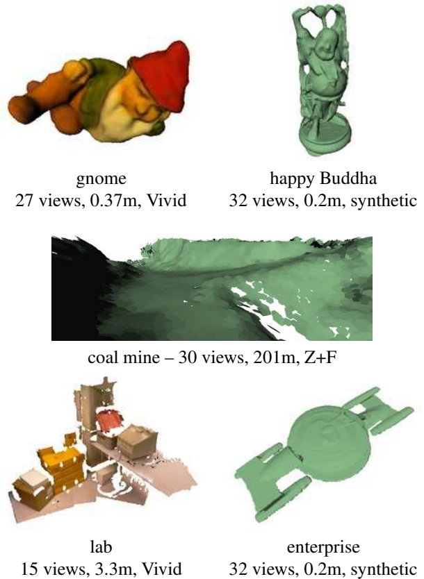
Figure 7. Example modeled scenes with number of views, scene size, and sensor used. Bottom right: The algorithm failed due to symmetry in the scene.
