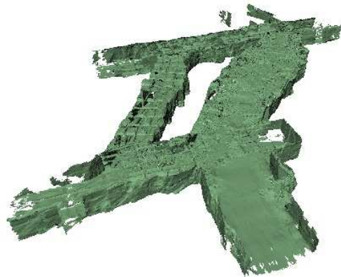
Figure 4: Perspective view of the automatically constructed mine model. The model consists of 23 separate views covering a region 43x42 m wide and 3 m high.
