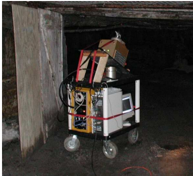
Figure 1: The cart-mounted Z+F laser scanner used in the data collection.
