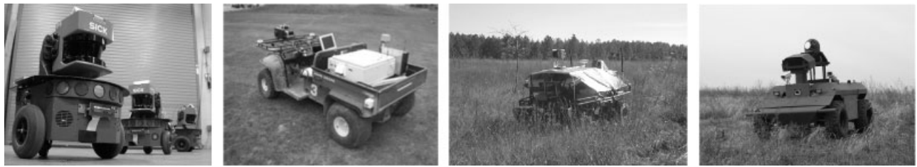
Figure 1. Some robots that currently use Field D^* for global path planning. These range from indoor planar robots (the Pioneers) to outdoor robots able to operate in harsh terrain (the XUV).
