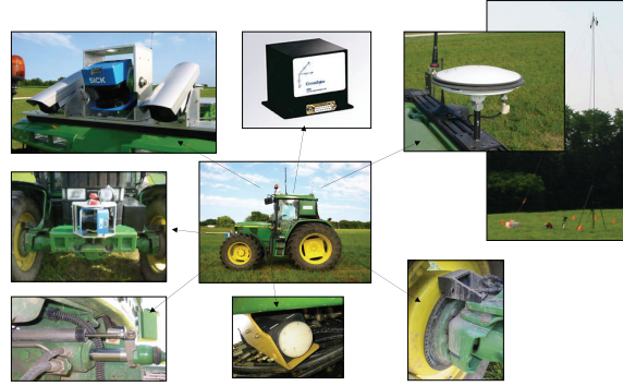
FIGURE 4.1. The autonomous tractor (center) and its sensors: a pair of high-resolution digital color cameras, two mechanically scanned SICK laser range finders, a steering potentiometer, a Doppler radar, four wheel encoders, a DGPS unit and three-axis optical gyro inertial measurement unit.
