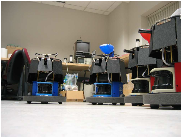
Figure 4.4: Four Obot robots developed by Botrics modified for use in paintball. The robots fire nerf balls out of paintball guns powered by compressed CO_2 . The black panels detect hits from other robots.
