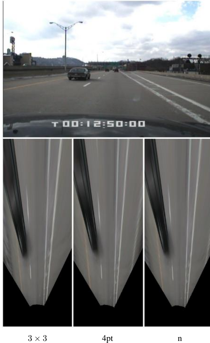
Figure 5: Top Down View Generation: A comparison of the performance of the 3 \times 3 parameterization, the 4pt parameterization, and the n parameterization in the fully calibrated setting. Each of the parameterizations is used to estimate the road plane, which is then used to generate a synthetic “Top Down View” by warping appropriately. The task is particularly difficult because of the lack of texture on the road and the oblique angle between the camera and the road plane. The image above is the first frame in an 800 frame movie. That movie clearly shows that the 3 \times 3 parameterization performs poorly. The n parameterization performs, if anything, slightly better than the 4pt parameterization.
