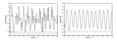
Figure 2: (Left) Control signal from open-loop learned controller. (Right) Resulting angle of one leg. The dashed line in each indicates which foot is grasping the bar at each time.
