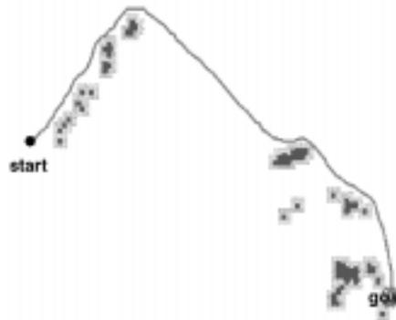
Fig. 16. Successful long traverse of the vehicle using Framed-Quadtree D\* through a terrain with obstacles to the goal. The dark rectangles are obstacles detected and avoided during the traverse. The shaded areas surrounding the dark obstacles are potentially dangerous zones.
