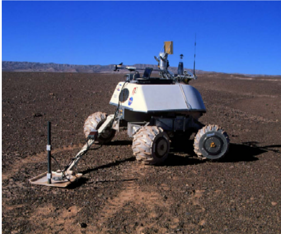
Figure 7.1 Robotic deployment of electromagnetic sensors (metal detector and magnetometers) in the Atacama Desert. Sensors are mounted on a non-metallic (polypropylene) platform, a distance away from the robot to minimize electromagnetic interference from the robot vehicle.
