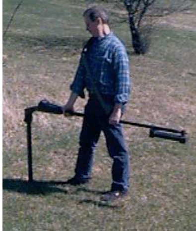
Figure 7.6 Ferex® magnetic gradiometer system for landmine and unexploded ordinance detection. Note the vertical probe, containing two co-aligned magnetic vector sensors. This unit was tested on various meteorite specimens in 1997, verifying that they had detectable magnetic fields. [Photo: Foerster Systems product brochure].
