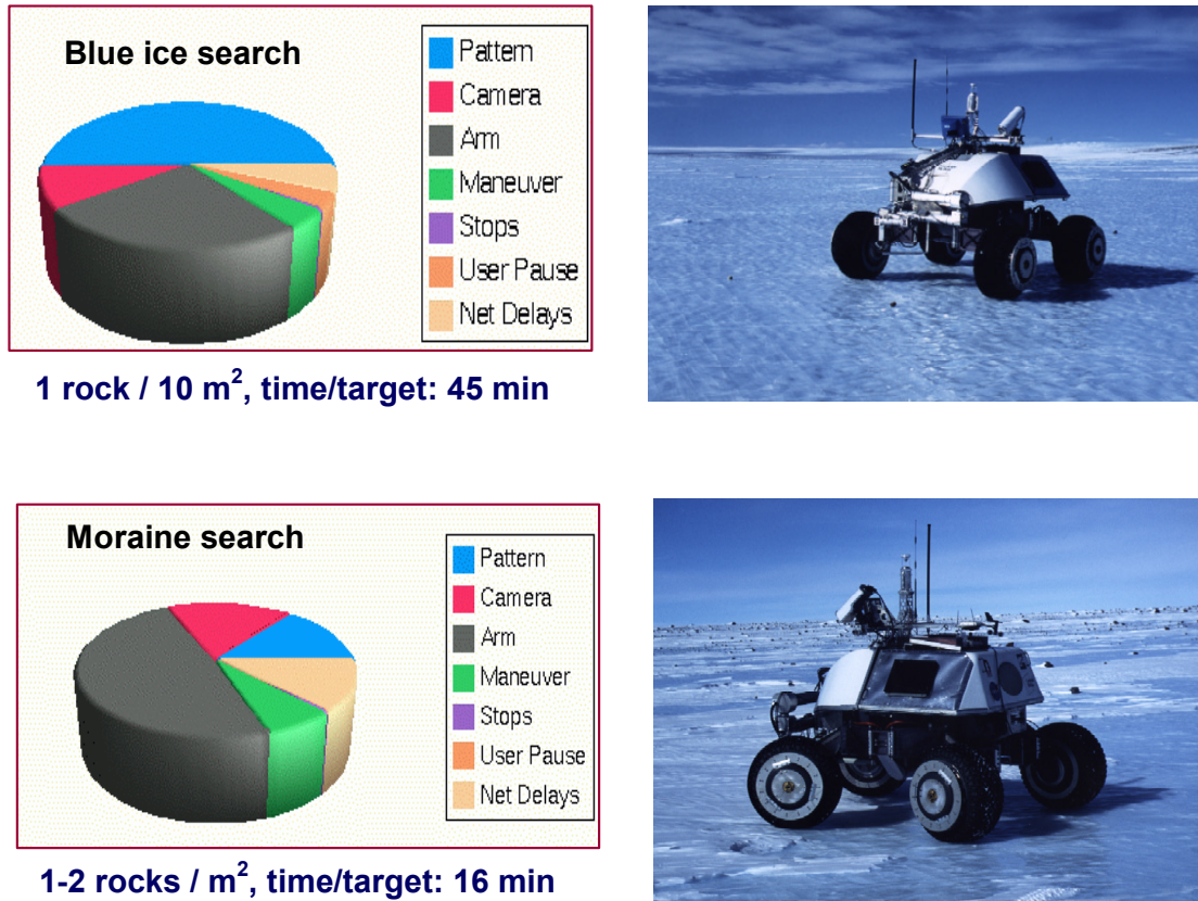
Figure 10.2 Breakdown of Nomad task times while searching for meteorites in Elephant Moraine, Antarctica. Most time is spent deploying the spectrometer sensor arm to acquire spectra, with some extra time spent maneuvering to bring Nomad into position. This illustrates the value of being able to dispense with spectral readings on those samples sufficiently well identified by the camera.
