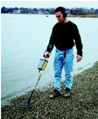
Figure 7.2 Pulse 8x® metal detector, a pulse induction type of eddy current sensor used to find meteorites in the Atacama Desert. [Photo: J.W.FisherMfg product brochure]
