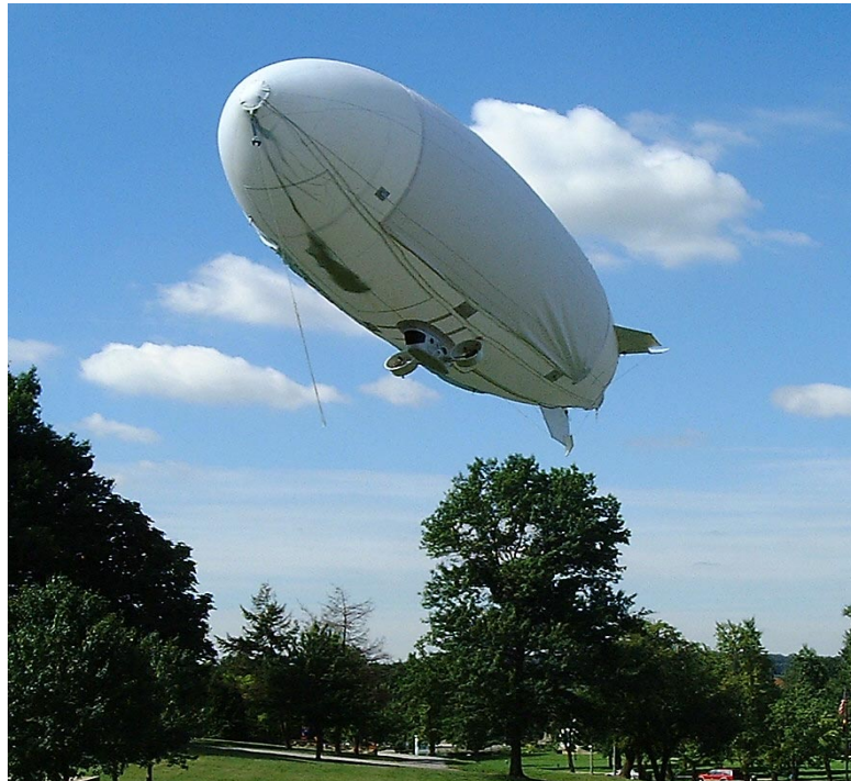
Figure 1: Nine meter (30 foot) airship during test flights in Pittsburgh, PA. This airship has been equipped with an on-board computer and a suite of navigational and environmental sensors. It will be used as a testbed for autonomy research and environmental sampling.
