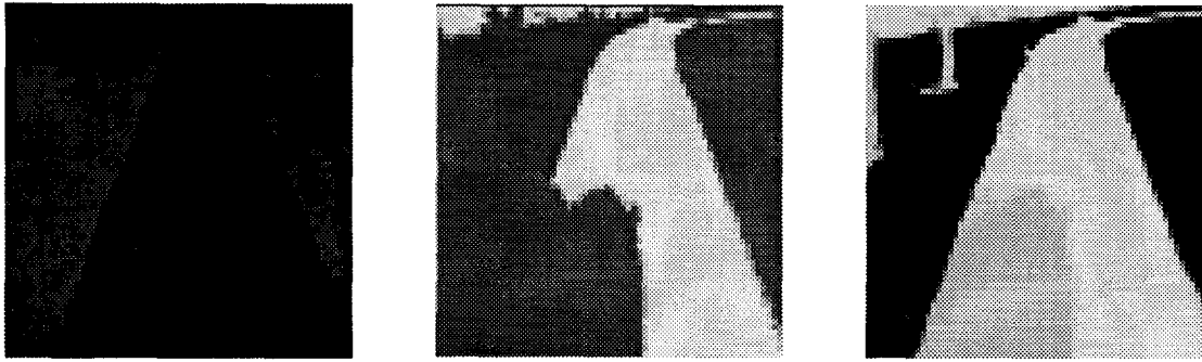
Figure 7. As the perceptron learns, its output better classifies road and non-road. The white pixels represent road, while the black represent off-road. Images shown perceptron output after 1, 3, and 6 training iterations.
