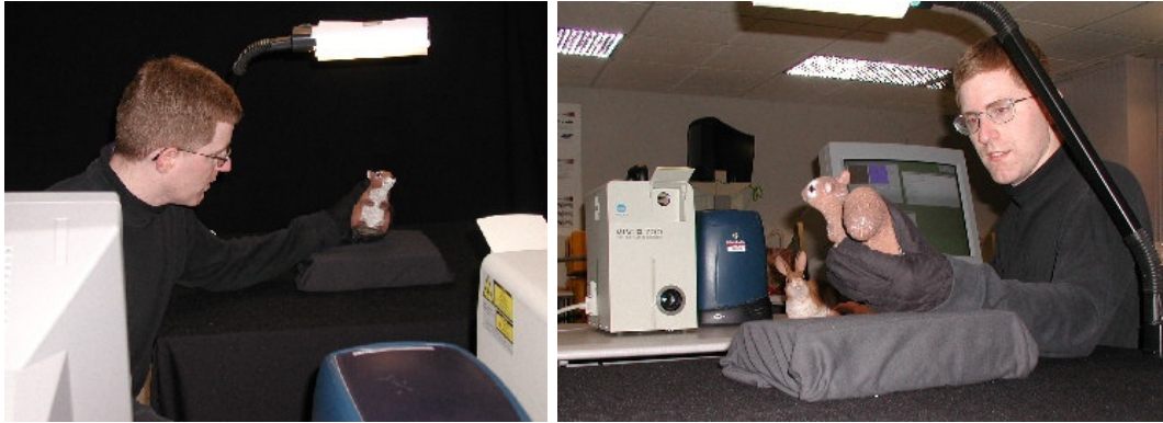
Figure 1.9: The hand-held modeling application. The object is held before the scanner while range images are obtained from various viewpoints (black clothes simplify the problem of background removal). The FAMUS system takes the range images and automatically produces a 3D model.
