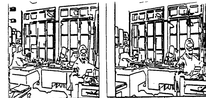
Figure 12: Polygonal approximation of the edge points of a stereo pair of an office room observed in position 1
