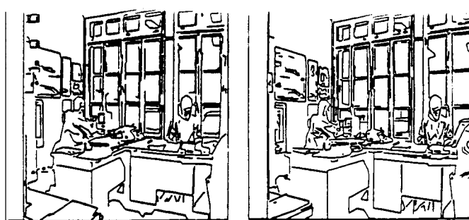
Figure 13: Polygonal approximation of the edge points of a stereo pair of the same office room observed in position 2
