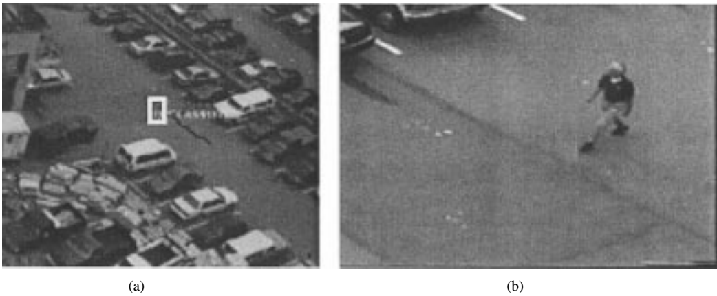
Fig. 10. Example of camera slaving. (a) Wide-angle view in which a person is detected. (b) A better view from a second camera, which has been tasked to intercept the person's estimated 3-D path.
