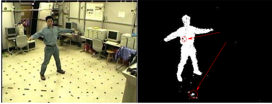
Figure 4. An example of a foreground image and its silhouette extracted by real-time background subtraction method. There are wrongly marked pixels in the silhouette image due to noisy original and background images.
