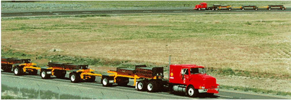
**Figure 1: Westrack automated pavement test vehicle**
