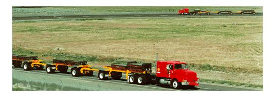
Figure 1: Westrack automated pavement test vehicle
