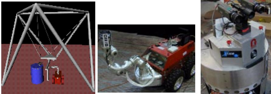
**Figure 2.** Experimental testbed consisting of crane, mobile manipulator, and roving eye robots.
