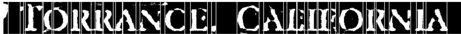
Fig. 10. Edges of peak in vertical projection profile. White lines indicate candidates of character segments.
