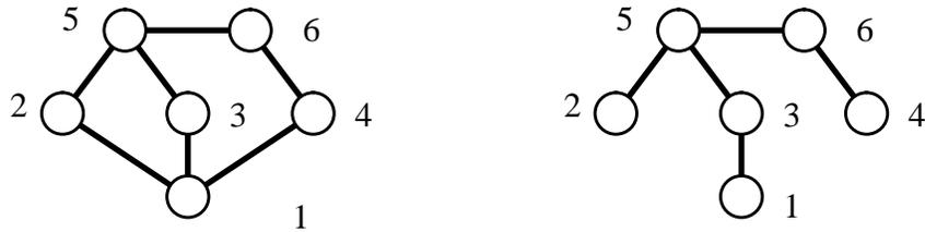
**Figure 49. Spanning tree for Stephenson III six-bar mechanism**
