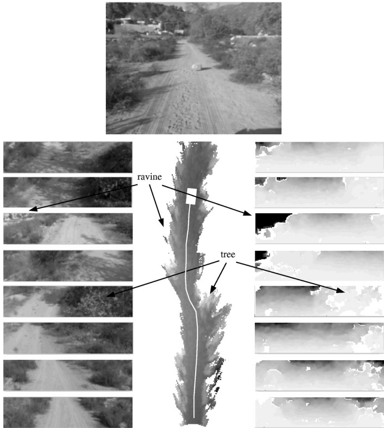
Figure 1: Road run with Ranger, covering about 200 meters. At top is an overview of the road travelled. Shown below are windows of attention from representative intensity images (left side), corresponding range images (right side), and a composite elevation map from the whole run (center). The white curve and rectangle on the elevation map represent the vehicle path and the vehicle itself at the end of the run. From Matthies et al. [1995, Obstacle Detection for Unmanned Ground Vehicles ]
