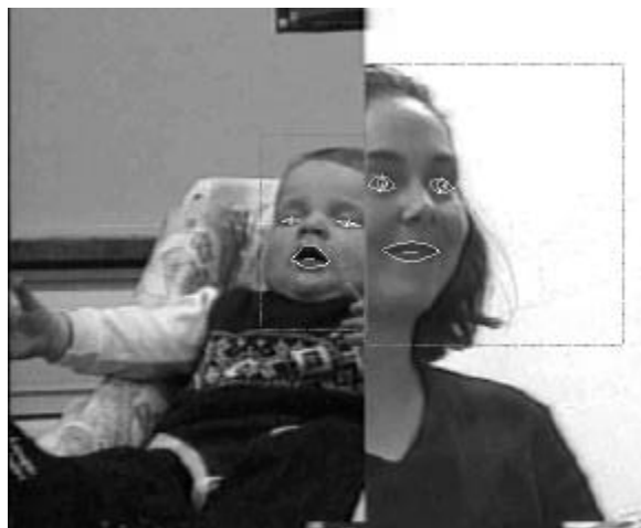
Figure 2. Automated face detection and facial-feature and eye tracking in image sequence obtained from synchronized cameras and split-screen generator.
