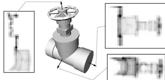
Figure 2. Some example spin-images for a CAD model of a valve
