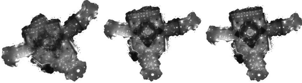
Figure 4: Three snapshots of the global alignment process using the *folding algorithm*, described in the text. Left: initial, bad alignment, using odometry only. Middle: intermediate result. Right: final global alignment.
