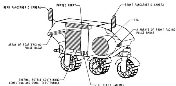
FIGURE 3 Cut out of Lunar rover
