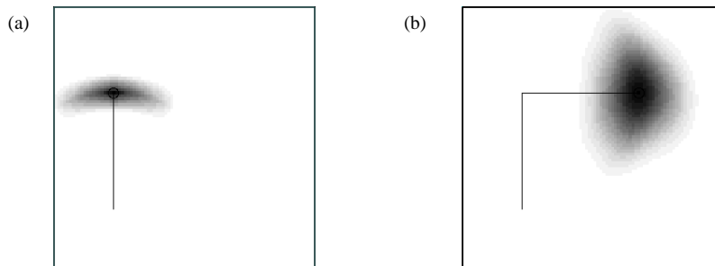
Figure 1. Probabilistic model of robot motion: Accumulated uncertainty after moving as shown: (a) 40 meter, (b) 80 meter.
