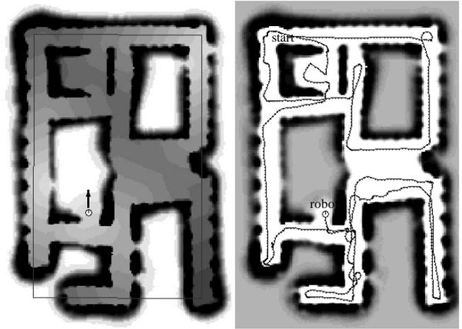
**Figure 5: Autonomous exploration.** (a) Exploration values, computed by value iteration. White regions are completely unexplored. By following the grey-scale gradient, the robot moves to the next unexplored area on a minimum-cost path. (b) Actual path traveled during autonomous exploration, along with the resulting metric map. The large black rectangle in (a) indicates the global wall orientation  $\theta_{\text{wall}}$ .
