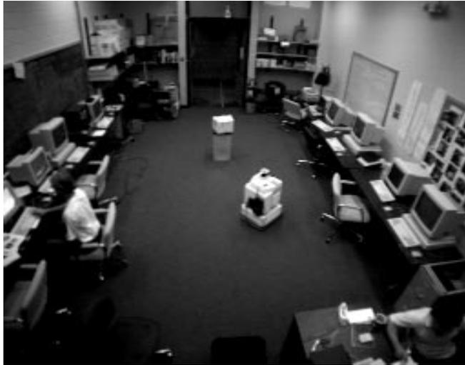
**Figure 9** The robot explores an unknown environment. Note the obstacle in the middle of the laboratory. Our lab causes many malicious sonar values, and is a hard testbed for sonar-based navigation. For example, some of the chairs absorb sound almost completely, and are thus hard to detect by sonar.
