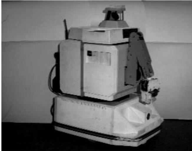
**Figure 2** The robot we used in all experiments described in this paper is a wheeled HERO-2000 robot with a manipulator and a gripper. It is equipped with two sonar sensors, one on the top of the robot that can be directed by a rotating mirror to give a full  $360^\circ$  sweep (24 values), and one on the wrist that can be rotated by the manipulator to give a  $90^\circ$  sweep. Sonar sensors return approximate echo distances. Such sensors are inexpensive but very noisy.
